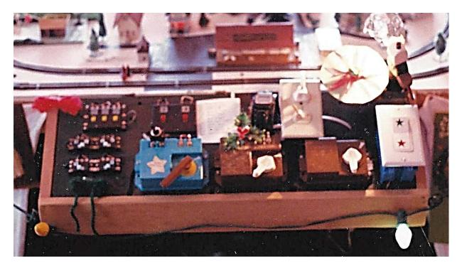
The two red switches and the three yellow switches on the upper left from that energize the siding in the harbor, the siding under Santa's Mountain, the shunt track siding between the outer and inner perimeter track and the freight yard track. It also controls the movement of the train on the freight yard track.
